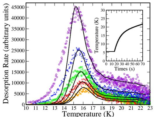
FIG. 2.— TPD curves of HD desorption after irradiation with H+D atoms on amorphous silicate with irradiation times of 15 ( $*$ ), 30 ( $\times$ ), 60 ( $\square$ ) 120 ( $+$ ) and 240 ( $\circ$ ) s. The solid lines are fits obtained using the rate equation model. The temperature ramps (shown in the inset) are identical for all the runs.
