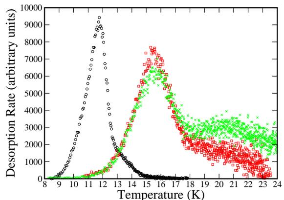
FIG. 1.— TPD curves of HD desorption after irradiation of HD molecules ( $\times$ ) and H+D atoms ( $\square$ ) on amorphous silicate. Also shown, for comparison, is HD desorption after irradiation with H+D atoms on polycrystalline silicate ( $\circ$ ).
