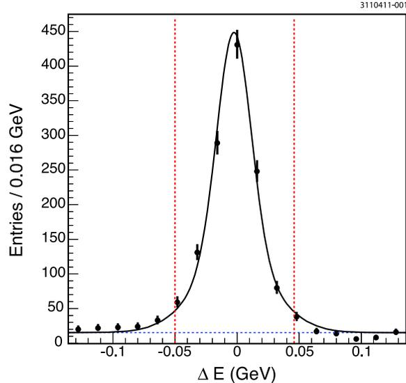
FIG. 1: Signal-side  $\Delta E$  distribution. The solid line shows the results of fitting with a double Gaussian to represent the signal plus a constant background (horizontal dashed line). The vertical dashed lines indicate the signal region.
