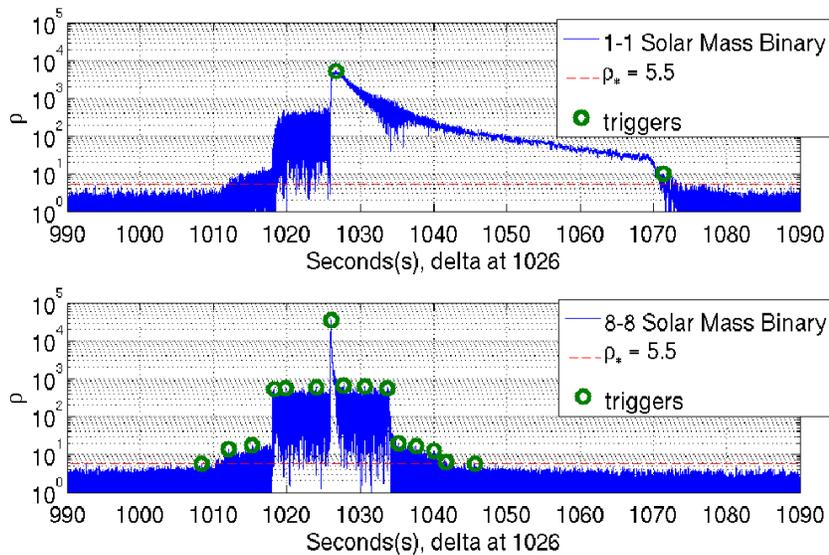
**Figure 1.** Matched filtering an impulse in Gaussian noise, colored based on the LIGO design sensitivity, using the CBC search with a single template. The result for two templates, top consisting of a binary of 1 solar mass objects, and bottom a binary of 8 solar mass objects. The red dashed line is the search threshold  $\rho_*$  of 5.5, and the green circles indicate the positions of the resulting triggers.
