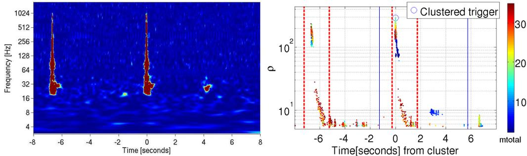
**Figure 2.** A pair of overflows in the length sensing and control system of H2. At left, a time-frequency representation [5]. At right, the effect of the transient on the production of unclustered triggers for the CBC search with total mass between 2 and 35 solar masses (dots), the 10 second clusters of these raw triggers (circle), the original Data Quality flags (dashed lines), and the expanded data quality veto after duration paddings are applied (solid lines).
