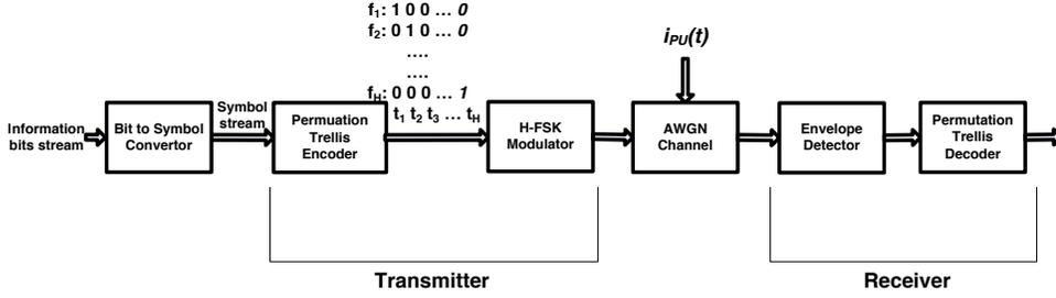
Fig. 2: Signal processing from transmitter to receiver
