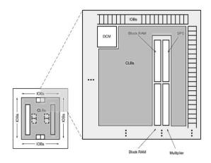
Fig.3 SPO on an FPGA
