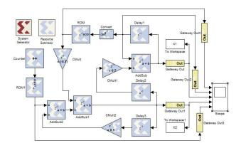
Fig.5 Simulink Model of a Driven Pendulum
