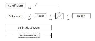
Fig.4 Pseudo Floating Point Bit Serial Multiplier
