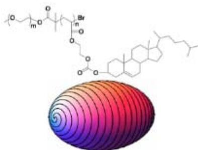
Ellipsoidal smectic polymer vesicles were formed from amphiphilic block copolymers in which the hydrophobic block is a smectic liquid crystal polymer.
