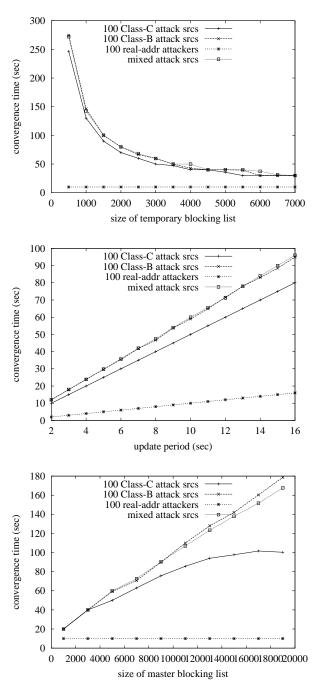
Fig. 4. Convergence time with respect to firewall configuration
