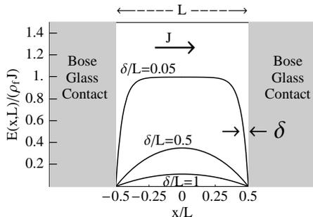
FIG. 1. A weakly irradiated channel (white region) where the flux liquid is sandwiched between two heavily irradiated Bose-glass contacts (shaded regions). A current  $J$  applied across the channel yields flux motion along the channel. The reduced field profiles given by Eq. (9) are shown for a few values of  $\delta/L$  and can be measured by a series of voltage taps.
