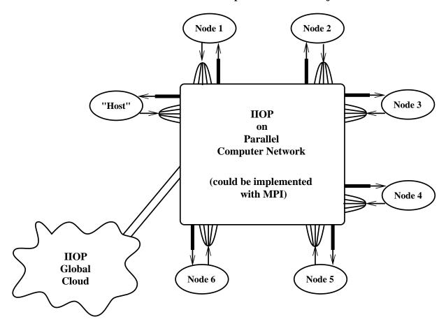
Figure 10: Each node of a parallel computer instantiated as a CORBA object.
