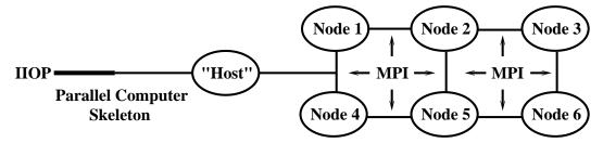
Figure 9: A Parallel Computer viewed as a single CORBA object in a classic "Host-node computing model.
