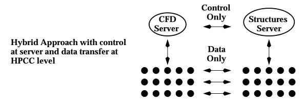
Figure 5(c): Hybrid approach to Linking Two Modules
