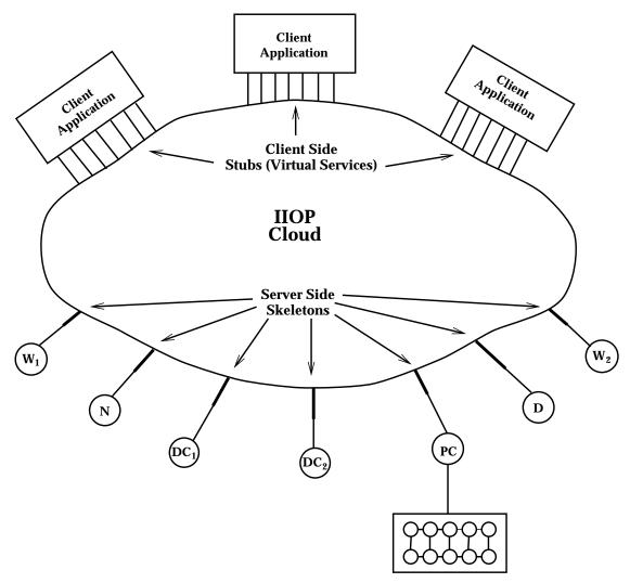
Figure 3: Pure CORBA architecture for the heterogeneous DcciS services of Figure 2. There is a similar Java version of this using RMI and JDBC with of course the linked application being restricted to Java code. CORBA and the analogous COM solution are cross-language solutions.
