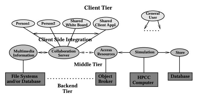
Figure 7: Collaboration in today's Java Web Server implementation of the three-tier computing model. Typical clients (on top right) are independent, but Java collaboration systems link multiple clients through object (service) sharing.
