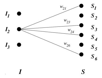
Figure 12: Abstract model of the server - a bipartite graph with two sets of nodes (I and S), with edge weights representing the time to retrieve  $P_S$  bytes from a server node. Figure shows admission control policy trying to determine if node  $I_2$  can accept a client request for sourcing a stream whose data is stored on nodes  $S_1$ ,  $S_3$ ,  $S_4$ , and  $S_6$ .
