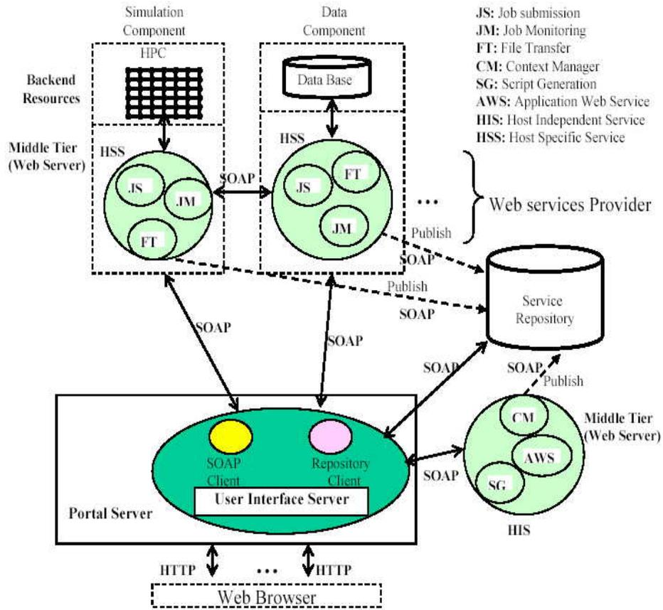
Fig. 1. Architecture of Web service-based computing portals.
