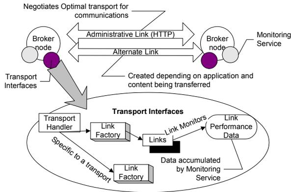
**Figure 2: Transport Framework – The bigger picture.**
