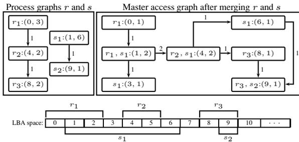
Figure 4: **Building the master access graph.** Vertices are defined by (start LBA, size of request). Since vertices  $r_1$  and  $s_1$  have overlapping LBAs,  $r_1$  is split into two vertices in the master access graph, one with size 1 and the other with the overlapping  $s_1$  blocks, starting at LBA 1 with size 2.
