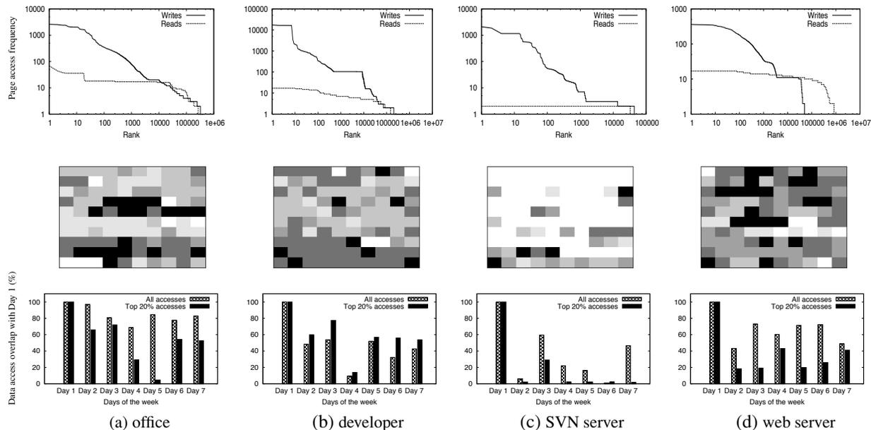
Figure 1: **Rank-frequency, heatmap, and working-set plots for week-long traces from four different systems.** The heatmaps (middle row) depict frequency of accesses in various physical regions of the disk, each cell representing a region. Six normalized, exponentially-increasing heat levels are used in each heatmap where darker cells represent higher frequency of accesses to the region. Disk regions are mapped to cells in row-major order.
