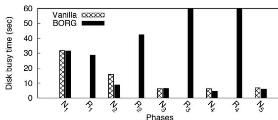
Figure 6: Disk busy times in various phases of the SVN server trace replay.  $R_i$  and  $N_j$  correspond to reconfiguration phase  $i$  and non-reconfiguration phase  $j$  respectively.  $R_3$  and  $R_4$  are beyond the y-axis range with values of 272 and 564 seconds respectively.
