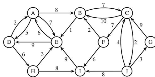
Figure 5: **Placing the master access graph.**  $C$  is the most connected vertex and is chosen for placement first. Next, vertex  $B$  is placed after vertex  $C$  since it is connected by an outgoing edge and has the highest weight of all the edges connected to  $C$ . Next, vertex  $G$  is placed before vertex group  $C \cup B$ . The final sequence of vertices from the lowest LBA to the highest is:  $L = [F, H, J, A, G, C, B, E, D]$ .
