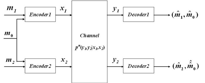
Fig. 1. Interference channel with common information.
