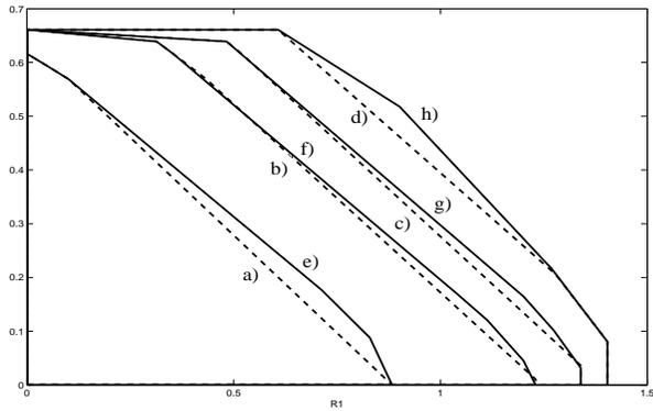
Fig. 3. Comparison of achievable rate region  $\mathcal{R}_T$  and  $\mathcal{R}_I$ .  $P_1 = 6, P_2 = 1.5, P_0 = 1, a_{12} = a_{21} = 0.74$ . Dashed lines are for  $\mathcal{R}_T$  while solid lines are for  $\mathcal{R}_I$ . a) and e) are for  $R_0 = 0.8$ ; b) and f) are for  $R_0 = 0.4$ ; c) and g) are for  $R_0 = 0.2$ ; d) and h) are for  $R_0 = 0$ .
