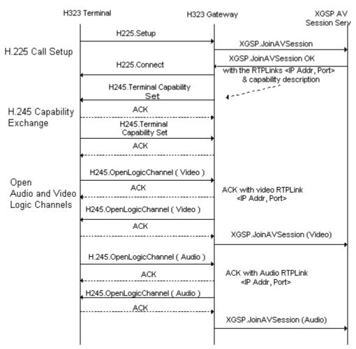
Figure 11. The translation of H.323 call into XGSP procedure
