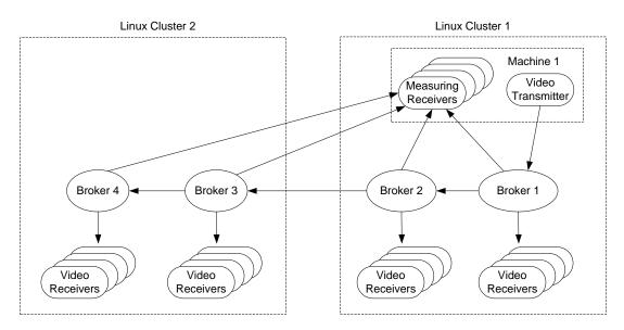
Figure 15 Single video meeting tests with four brokers
