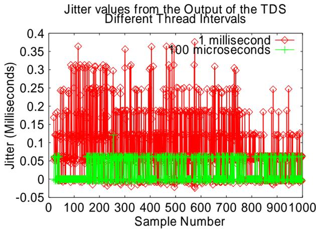
**Figure 18: Jitter values from the TDS output for different thread intervals (Trans-Atlantic)**
