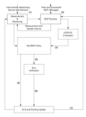
Fig. 3. BMP Control Mechanisms
