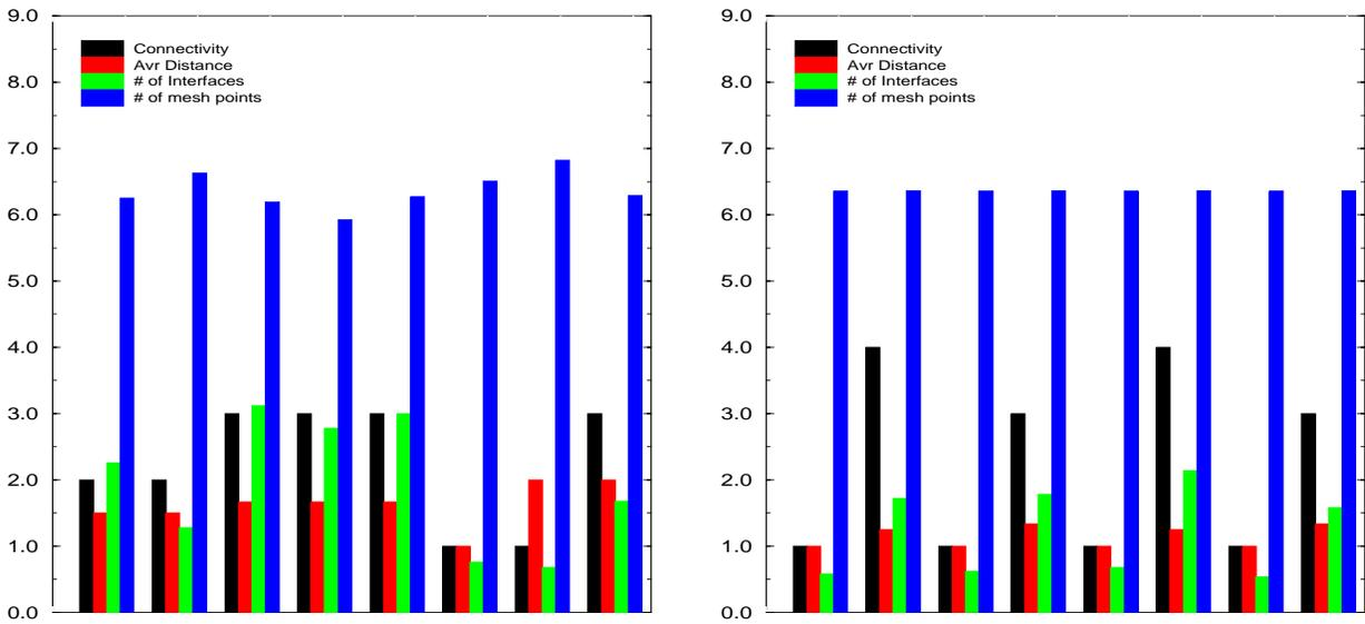
Figure 8: Bar charts that depict the tradeoff between load balance and communication for GA (left) and RSB (right). Each chart consists of eight groups (x-axis) of four bars that depict connectivity, average distance, number of interfaces divided by 25, and total number of nodes divided by 250 per submesh. Y-axis has no metric.
