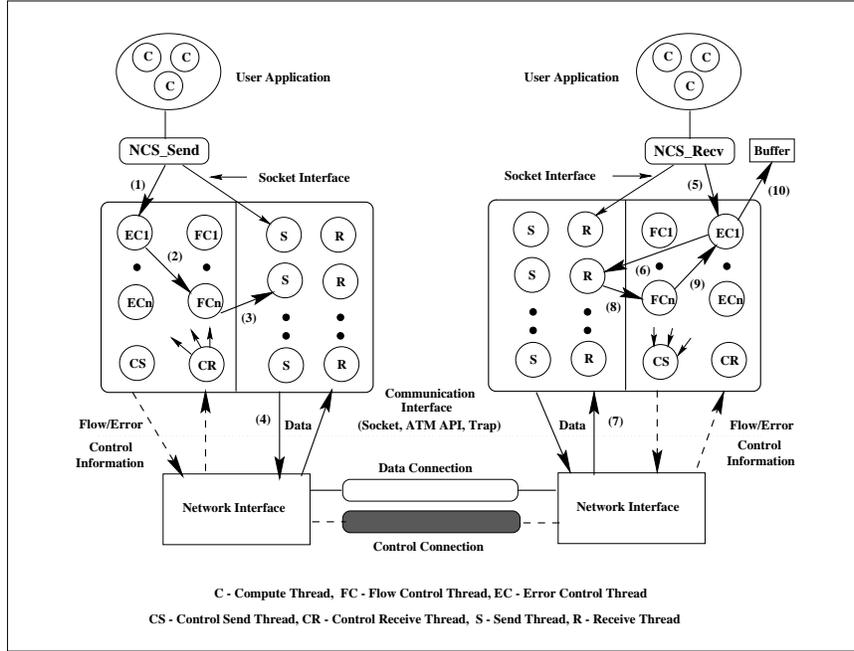
Figure 4: Point-to-Point Communication in the NCS Environment
