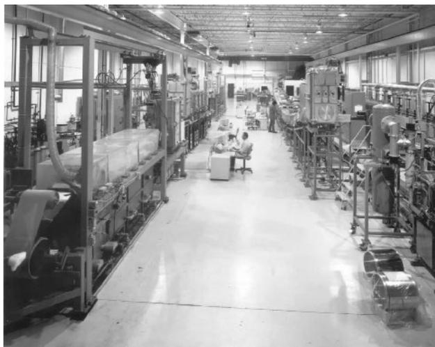
**Figure 12.27** A photograph of the Energy Conversion Devices, Inc. 2-MW plant showing all four front-end roll-to-roll machines for washing, back reflector sputter deposition, PECVD deposition (right-hand side) and TCO deposition [185]
