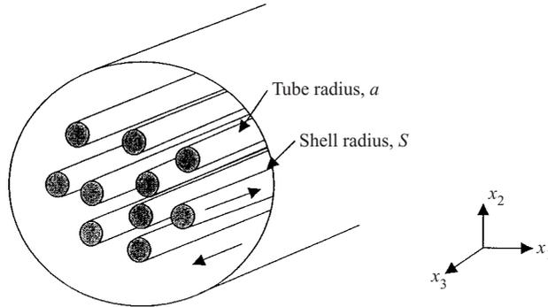
FIGURE 1. A schematic representation of a hollow-fibre contactor.
