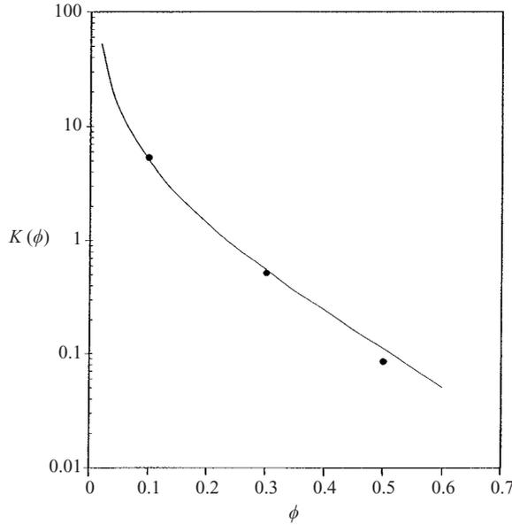
FIGURE 4. The non-dimensional permeability  $K$  as a function of  $\phi$  for random arrays of tubes. The filled circles are the results of numerical simulations and the solid line the effective-medium approximation.
