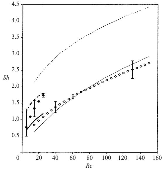
FIGURE 13. Comparison with the experimental results. The filled circles and diamonds are from the correlation by Prasad & Sirkar for  $\phi = 0.1$  and  $0.4$ . The thick and thin solid lines are the theory predictions for  $\phi = 0.1$  and  $0.4$ , each with  $F = \exp[-(\delta/\delta_0)^2]$ . The dashed thick and thin lines correspond to  $F = 1$ .
