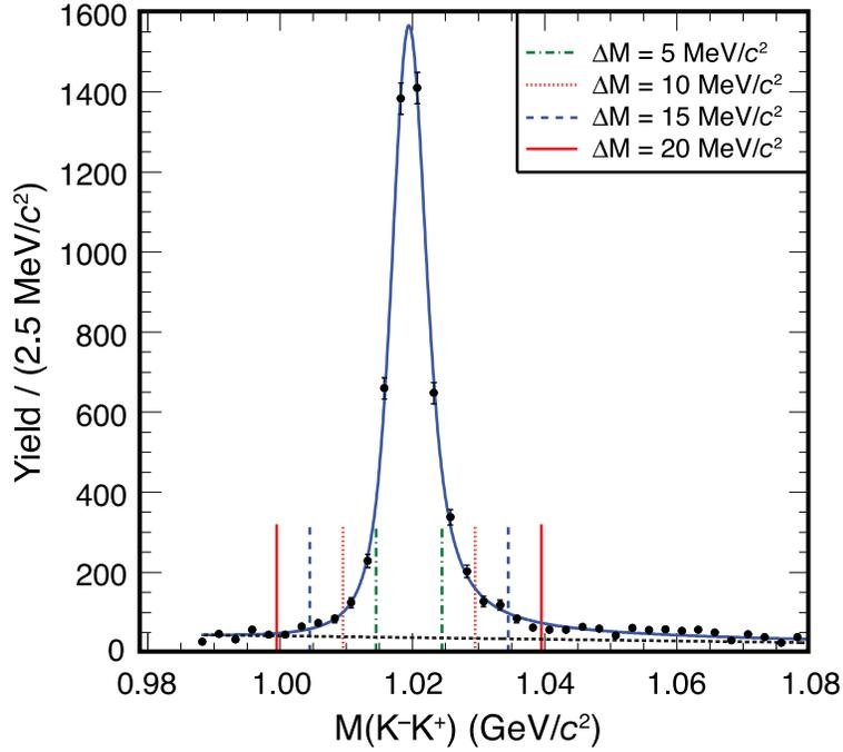
**Figure 1:** Dalitz plot projections for  $K^+K^-$  invariant mass in  $D_s^+ \rightarrow K^+K^-\pi^+$  from the CLEO Collaboration [7]. The signal is extracted individually in each mass bin, thus there is no background. The data are fit with a Breit-Wigner signal function for the  $\phi$  convoluted with a Gaussian for detector resolution and linear representation of an S-wave component (dashed line). The solid curve shows the sum. (Only the data is ascribed to CLEO, the fits have been added.)
