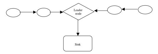
Figure 3: Chain based organization in a sensor network. The ovals indicate sensors and the arrows indicate the direction of data transmission.
