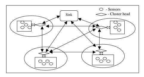
Figure 2: Cluster based sensor network. The arrows indicate wireless communication links.
