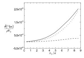
FIG. 9. The predictions of the mass flux term  $\hat{\theta}_2^{2,1}(m)$  from the detailed kinetic theory (solid line) and two the limiting theories (dotted line: LV approximation; dashed line: SV approximation).
