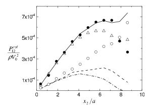
FIG. 13. Results for the total collisional contribution to the shear component  $P_{12}^{\rm col}$  [see Eq. (30)]. Filled circles: numerical simulations; solid line: detailed kinetic theory; dashed line: Jenkins and Mancini (Ref. 28) theory; dashed-dotted line: Lathouwers and Bellan (Ref. 33) theory; open circles: LV approximation added to the Jenkins and Mancini theory, triangles: Grad approximation added to the results given by open circles.
