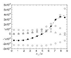
FIG. 14. Filled circles and dashed line represent, respectively, the lhs and rhs of the balance equation [see Eq. (31)] for  $T_{11}^1$ . Open symbols represent various terms on the rhs of Eq. (31). Circles represent the first term, squares the second and third terms, triangles the fourth term, and diamonds the fifth term.
