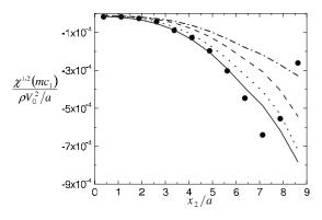
FIG. 12. Results for the source of momentum in the absence of mass exchange, i.e.,  $\chi^{1,2}(mc_1)$ . Filled circles: numerical simulations; solid line: detailed kinetic theory; dotted line: LV approximation; dashed line: Jenkins and Mancini (Ref. 26) theory; dashed-dotted line: Lathouwers and Bellan (Ref. 33) theory.
