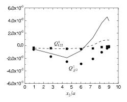
FIG. 15. Two selected components of heat flux tensor ( $Q_{122}^1$  and  $Q_{jj2}^1$ ). Symbols represent results from numerical simulations and lines represent predictions by the closure relation given by Eq. (69).
