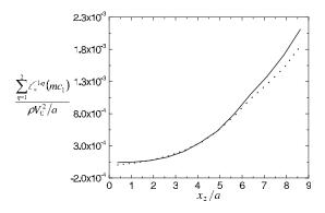
FIG. 11. A comparison of the momentum source due to conversion of species obtained using the detailed kinetic theory (solid line) with the limiting theory (dotted line) which assumes that both species are moving simply with their average velocities (LV approximation).
