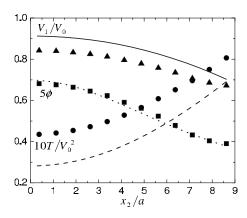
FIG. 1. The profiles of volume fraction, nondimensional velocity, and particle phase temperature for  $\langle \phi \rangle = 0.1$ ,  $\alpha = 0.5$ ,  $\gamma = 1$ , St=50, and N=191. Filled symbols and lines represent, respectively, numerical simulations and simple kinetic theory.
