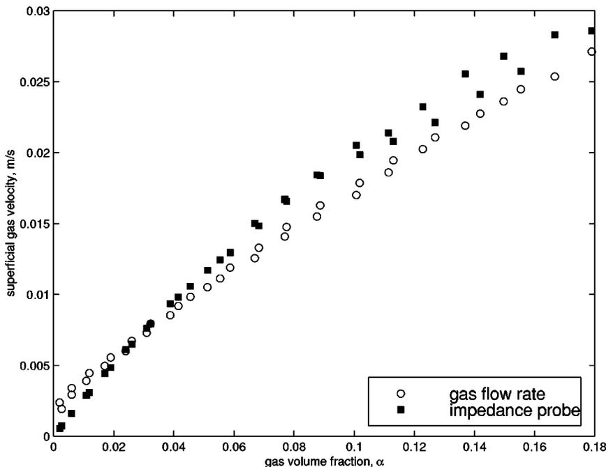
FIG. 12. Superficial gas velocity as a function of mean gas volume fraction. The size of the symbols denotes approximately the magnitude of the experimental error.
