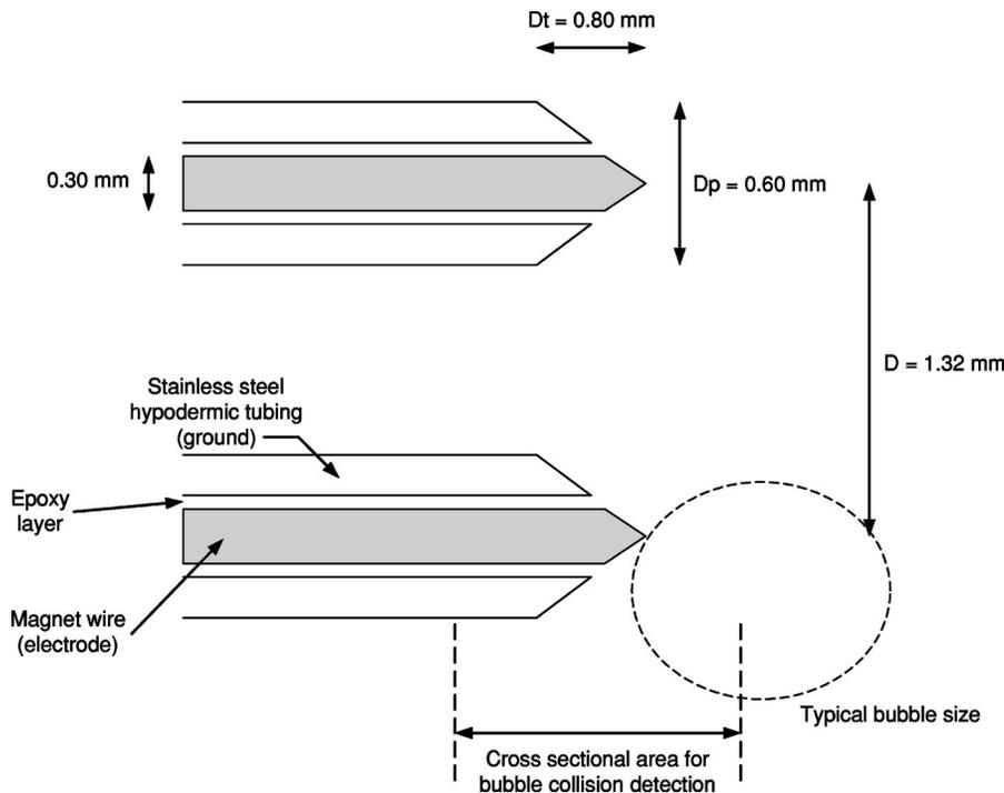
FIG. 1. Sketch of the dual impedance probe.
