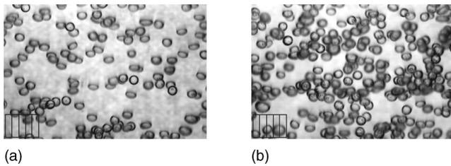
FIG. 5. Photographs of the flow for two typical gas volume fractions. The bubble size is nearly monodispersed for both cases. The spacing in the grid, shown in the lower-left corner, is 1 mm. (a)  $\alpha=0.02$ , (b)  $\alpha=0.05$ .
