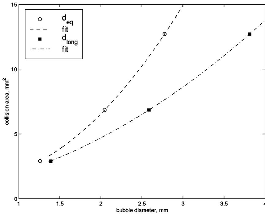
FIG. 9. Measured collision area as a function of the bubble equivalent diameter  $d_{eq}$  and bubble's long axis  $d_{long}$ . Lines show the fit to the measurements.
