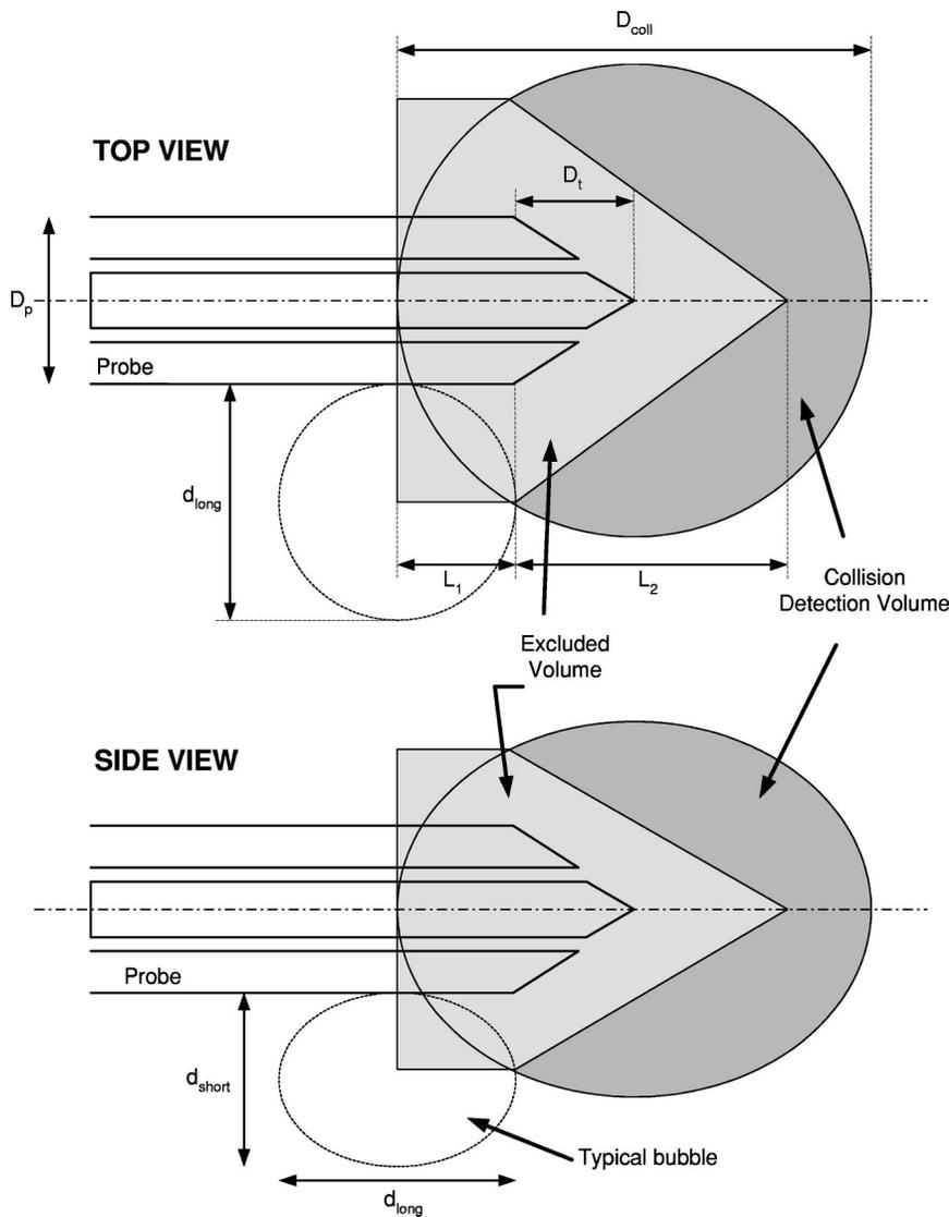
FIG. 8. Sketch of the geometry of the probe excluded volume and bubble collision detection volume.
