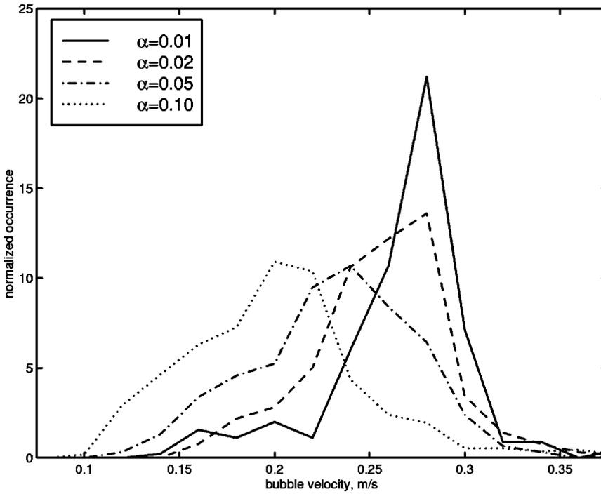
FIG. 13. Normalized bubble velocity probability density function for four typical gas volume fractions. The width of the bins is 0.02 m/s.
