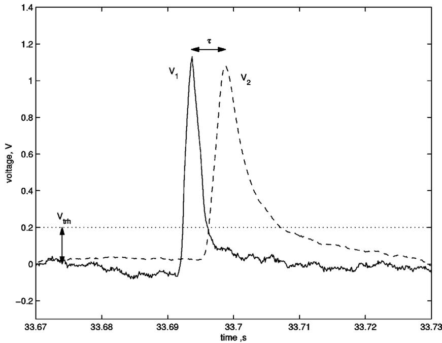
FIG. 3. Typical voltage signal resulting from a bubble passing near the tip of the probe. The solid line denotes the signal obtained from the leading probe, the dashed line shows the signal from the trailing probe. The dotted line denotes the voltage threshold level. The voltage threshold and the time delay between signals are also shown.
