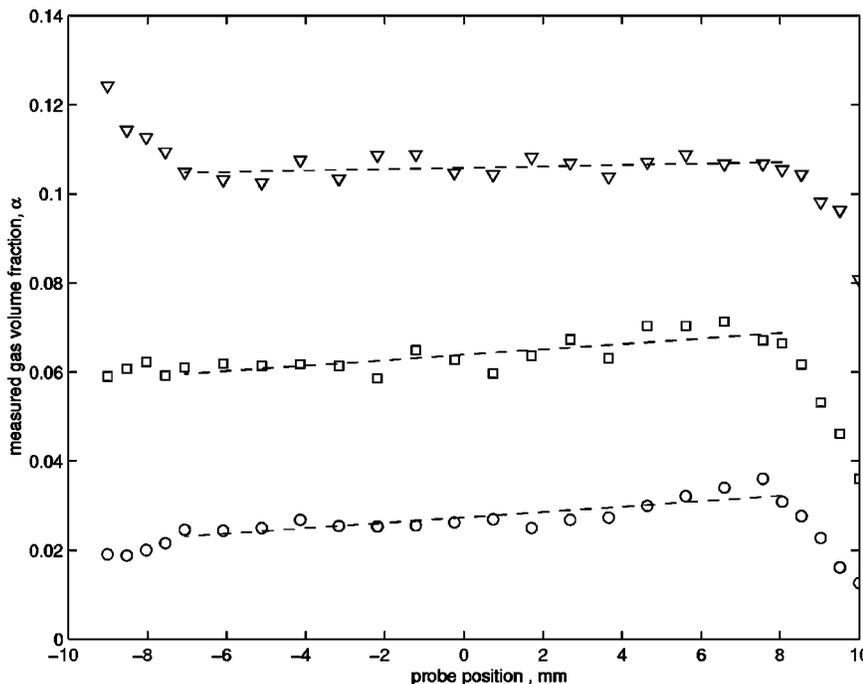
FIG. 10. Gas fraction profiles for three typical hold ups. ( $\circ$ ),  $\alpha=0.02$ ; ( $\square$ ),  $\alpha=0.05$ ; and ( $\nabla$ ),  $\alpha=0.10$ , for a channel inclination of  $\theta=5^\circ$ . The lines show best linear fits of the data excluding the near-wall regions.
