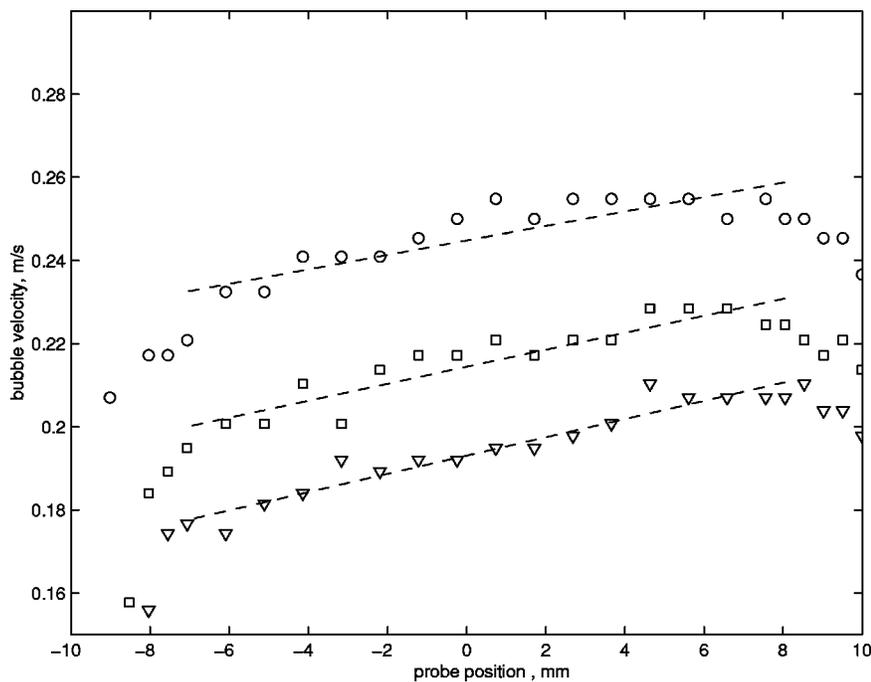
FIG. 14. Bubble velocity profiles for three typical hold ups. ( $\circ$ ),  $\alpha=0.02$ ; ( $\square$ ),  $\alpha=0.05$ ; and ( $\nabla$ ),  $\alpha=0.10$ , for a channel inclination of  $\theta=5^\circ$ . The lines show the linear best fits.
