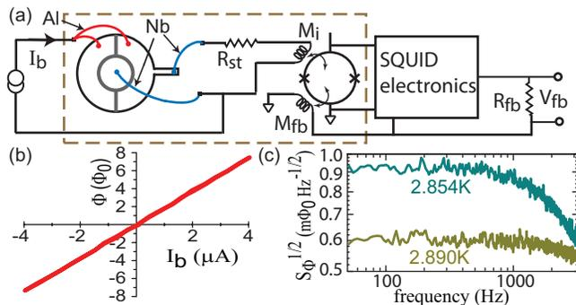
FIG. 2: (Color online) (a) Voltmeter circuit schematic; portions outside dashed box are at room temperature. (b) Flux coupled to SQUID vs.  $I_b$  at 4.2 K. (c) Flux noise spectra above and below  $T_c^{NbGe}$ , both measured with  $I_b = 0$ ,  $H_a = 0$ .
