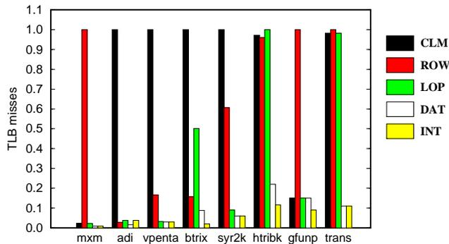
Figure 16: TLB misses. The results shown are normalized according to the worst-performing version for each program. The impact of our approach on TLB misses is very significant. For the first four codes in our experimental suite, our approach eliminates almost all TLB misses, confirming our argument on processor locality in Section 4.4.
