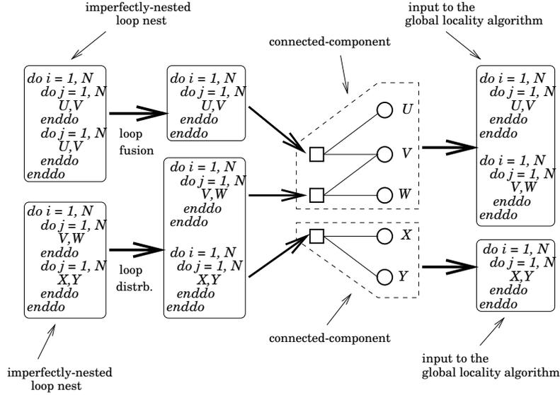
Figure 3: Example application of locality optimization algorithm.
