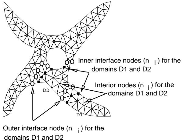
Figure 3: The components of the decomposed discrete PDE problem based on the splitting of the mesh or grid  $D^h$  used numerically. This discrete mesh is partitioned by interface nodes (shown as circles) into discrete subdomains  $D_i^h$
