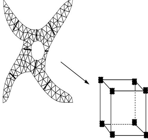
Figure 6: A problem partitioning and allocation methodology for PDE solvers on MIMD machines based on the domain decomposition approach.
