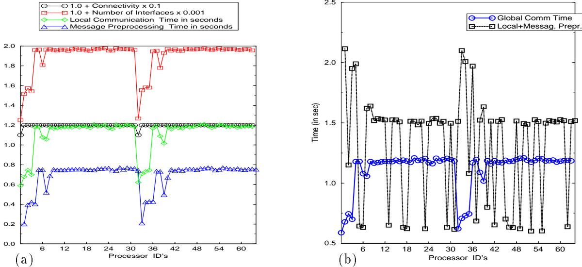
Figure 19: Relationship between the number of interfaces and message passing overhead of the Jacobi-SI method on the nCUBE II with 64 processors and Model Problem A, using the (a)  $1 \times Q$  block partition algorithm, and (b) the global and local communication.
