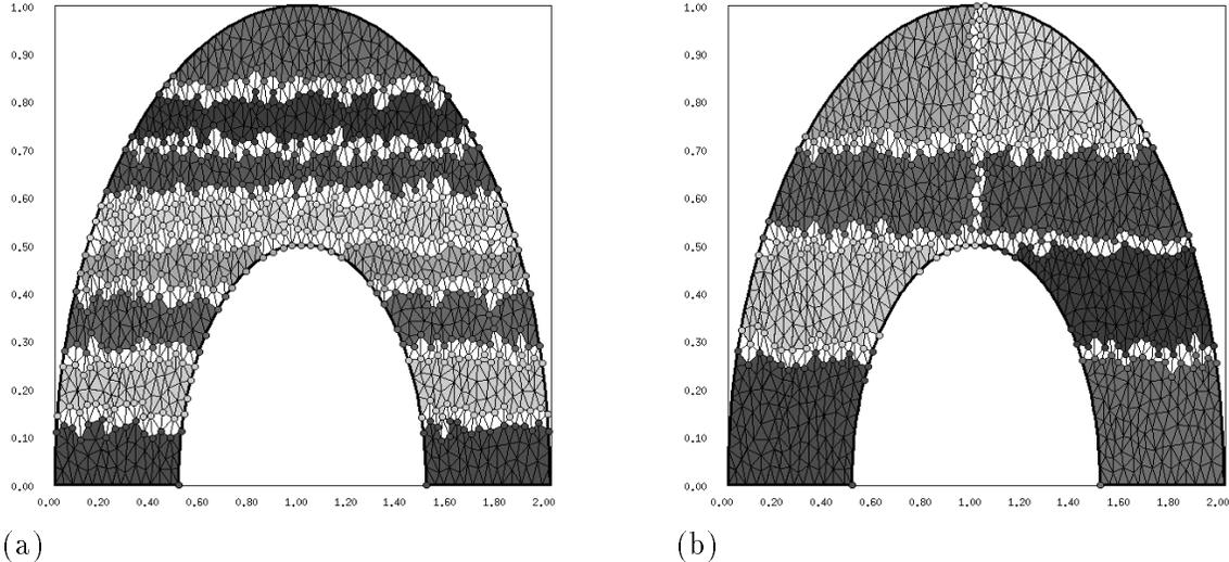
Figure 4: (a) Partition of a discretized semi-annulus domain using the  $1 \times 8$  partitioning algorithm. (b) Partition of a discretized semi-annulus domain using the  $2 \times 4$  partitioning algorithm.
