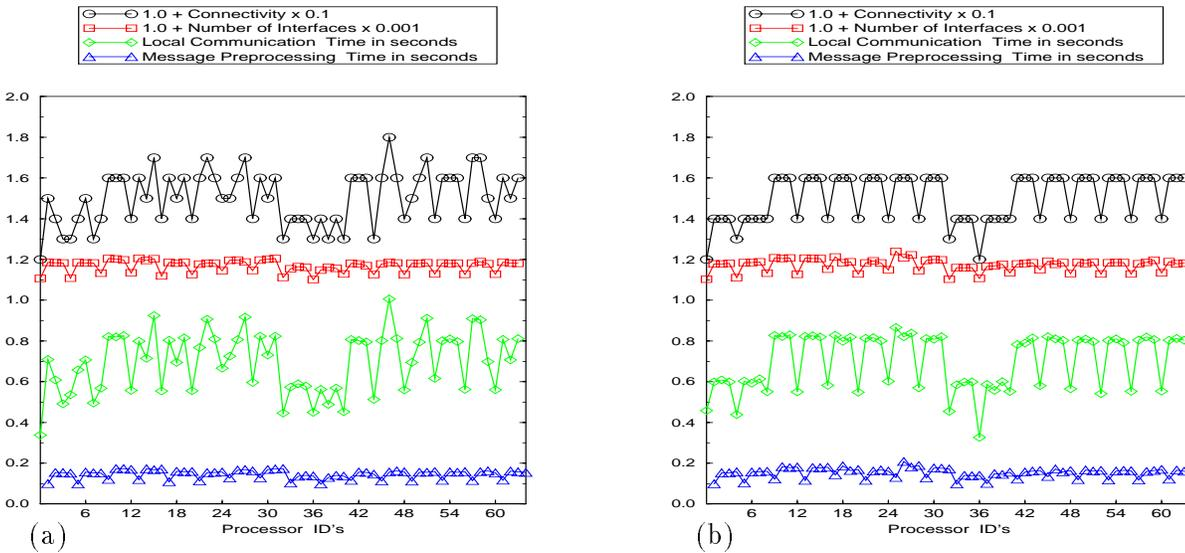
Figure 18: Relationship between the connectivity and message passing overhead of the Jacobi SI method on nCUBE II with 64 processors and Model Problem A for (a)  $P \times Q$  block partition and (b)  $Ext\_P \times Q$  block partition.
